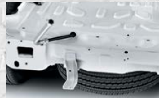
SPARE WHEEL ACCESSIBLE FROM THE REAR AND COMPATIBLE WITH MOST CONVERSIONS (OPT. 980)
